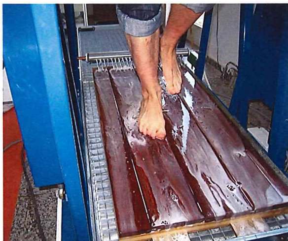
Fig. 2: Wet deck boards during the test on the ramp test
