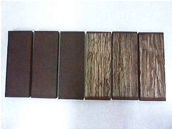
Figure 1: Surface of representative test specimens before (left side) and after (right side) 4 weeks of QUV weathering
